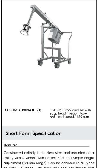
of pots. Equipped with tube and tool for mixing and blending soups and other semi-liquids or liquids. Safety device allows the machine to start only when in working position. All components of tube and head are in stainless steel and dishwasher safe (excluding bearings). 1 speed: 1650 rpm. The touch button control panel has IP65 protection with low voltage level.
